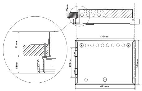
Figure 8. Flush mounting holes.
