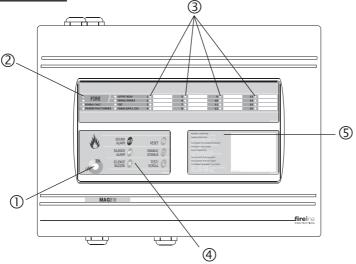
$\bigcirc$  - Switch for changing over between Access Levels 1 and 2. In OFF position (Access Level 1) only the SILENCE with the subscripts button is active and in ON position (Access Level 2) all buttons are active.
