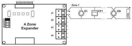
Figure 26. Example for Instant Action Mode Programming.
